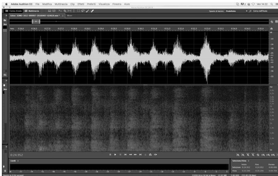
Fig. 1. Screenshot of Adobe® Audition™ CS6. Waveform (upper part) and spectral display (lower part) of an audio file.
