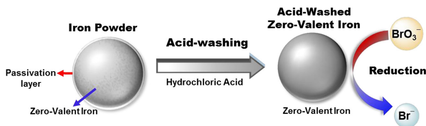
Fig. 1. Schematic illustration of acid-washed zero valent iron for reductive removal of bromate.
