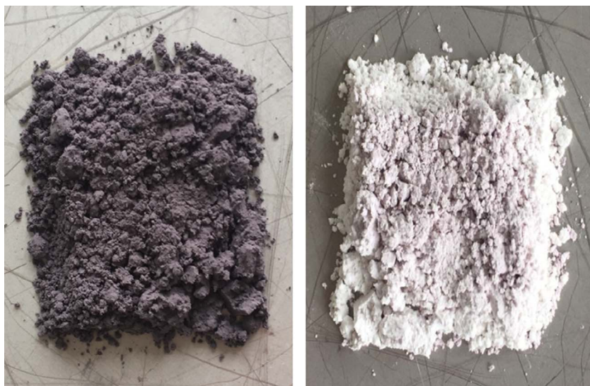
Fig. 1. Color of thermochromic powder below and above transition temperature: left is below 31 °C, right is above 31 °C.
