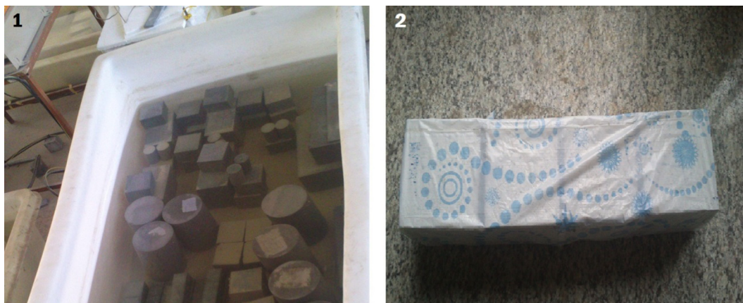
Fig. 1. Curing condition: 1) water curing, 2) under plastic cover.
