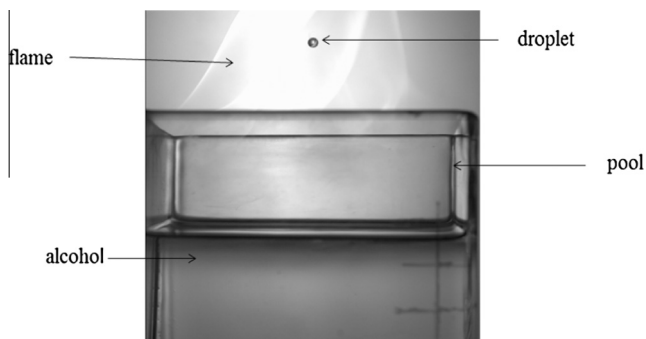
Fig. 2. The falling droplet and flame on the burning fuel.
