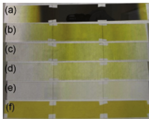
Fig. 1. Photographs of YH:O thin films deposited on glass substrates at total gas pressures of (a) 0.4, (b) 1.2, (c) 2, (d) 3 and (e) 6 Pa. The films were deposited using a stationary carrier. (f) Representative YH:O thin films obtained at a deposition pressure of 0.8 Pa by oscillating the substrate carrier in front of the Y target.
