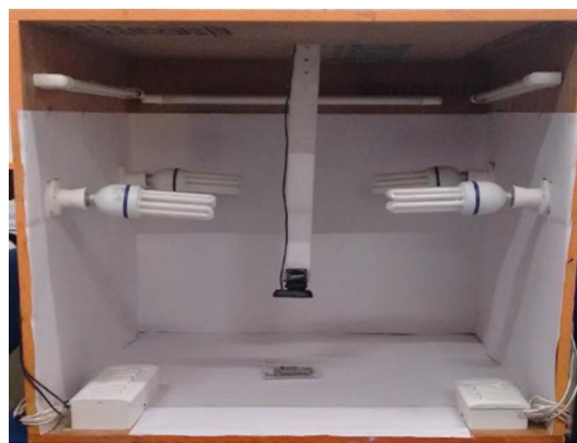
Fig. 1. Setup for image acquisition of the potato chips sample.
