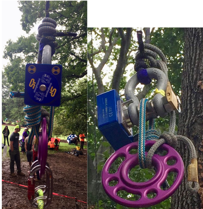
Fig. 1. Views of the load shackle incorporated into the event setup from the side (left) and front (right) show (from top to bottom in each image) the haul rope, the load shackle, and the rigging hub. The bottom of the left-hand image also shows two carabiners connecting ascent lines to the hub.
