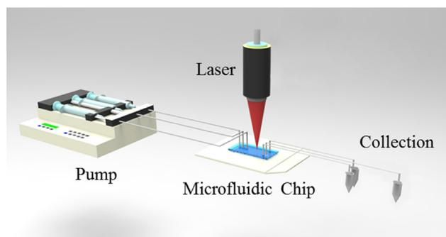
Fig. 1. Schematic of the photothermal effect based droplet microfluidic system for PCR application.
