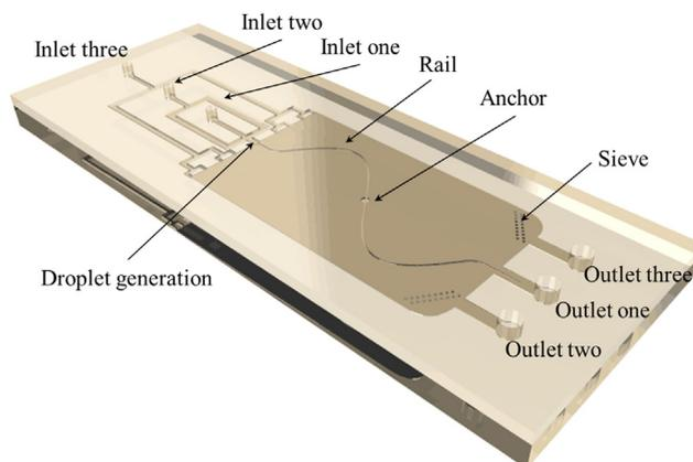
Fig. 2. Illustration of the microfluidic chip design.
