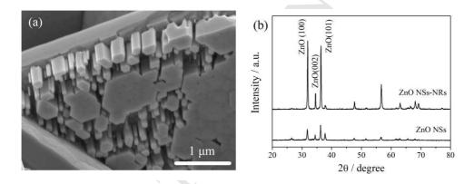
Fig. 1 FE-SEM micrographs (a), TEM (inset figure of (a)) and XRD (b) of ZnO NS-NRs prepared without the  $TiO_2$  intermediate layer, 0.6 M  $Zn(CH_3COO)_2$  seed precursor solution, 8 h hydrothermal treatment
