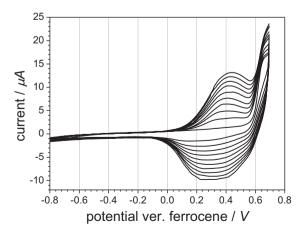
Fig. 2. Cyclic voltammetry of 6T3PhA; potential sweep rate 50 mV/s; 1 mM monomer solution in 0.1 M Bu<sub>4</sub>NPF<sub>6</sub> in CH<sub>2</sub>Cl<sub>2</sub>.
