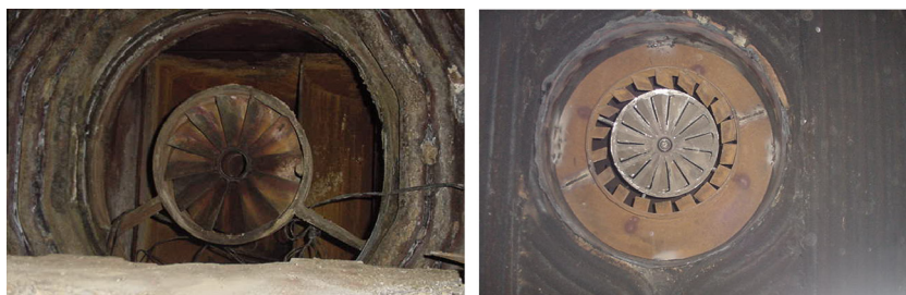
Fig. 1. Real burner with an old diffuser without swirler ring and a similar burner with the new design already in place.
