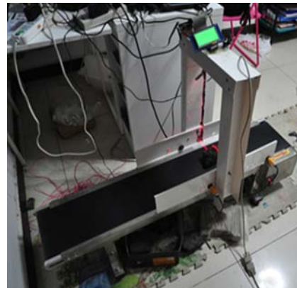
Fig. 1. Diagram and photograph of the coal-gangue separation system used in this study. a. Schematic diagram, b. Experimental equipment.
