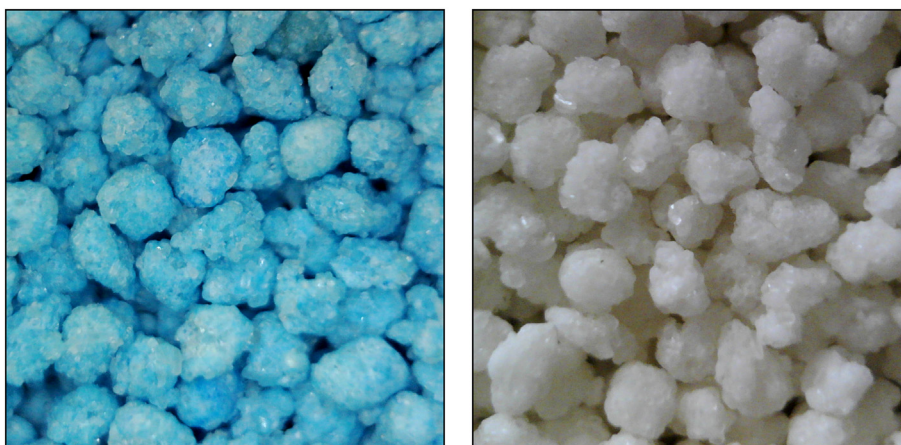
Fig. 1. Blue and white TAED particles used in the experiments (size fraction 400–500 microns).
