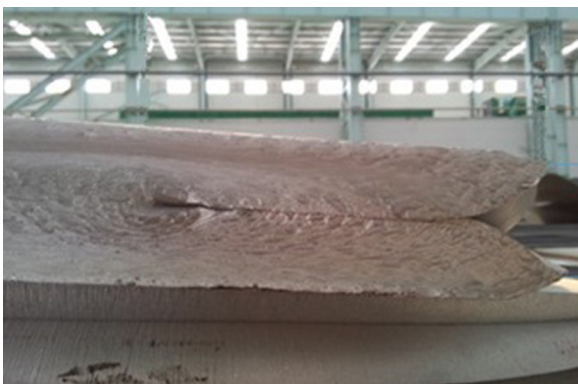
Fig. 2 – The crocodile mouth after multi-pass of rolling [2].
