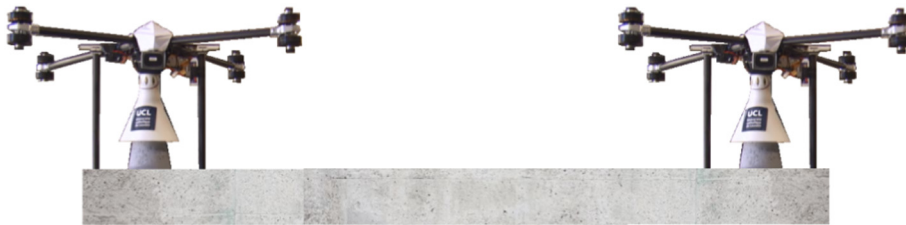
Fig. 2. Transportation of a long concrete beam by two synchronized UAVs.
