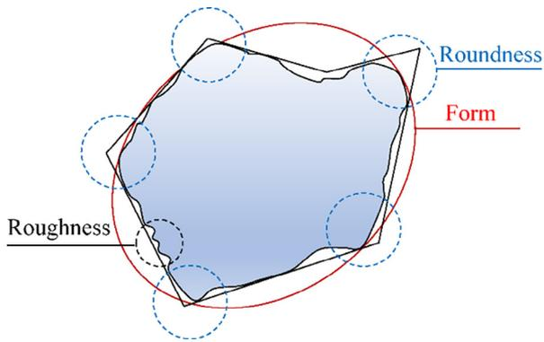
**Fig. 1.** Classification of particle shape features on three different scales (from Barret [8] and ISO [9]).
