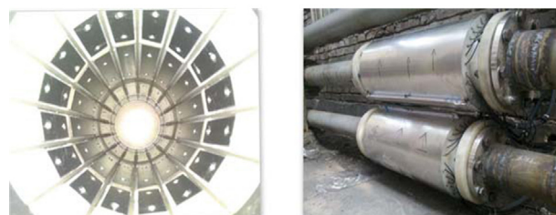
Fig. 3. Capacitance sensors for gas–solid two-phase flow measurement.
