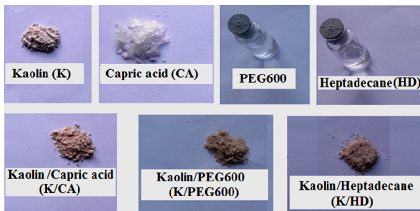
Fig. 1. Photograph images of pure kaolin, pure CA, pure PEG600, pure HD and the fabricated K/CA, K/PEG600 and K/HD composite PCMs.
