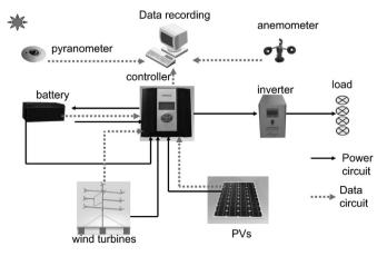
Fig. 2. Sketch map of the data acquisition system.
