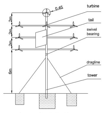
Fig. 1. Structure of the multi-turbine wind power system.
