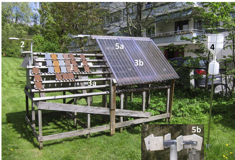
Fig. 1. The ICP-materials station (no. 21, Appendix A) located in the urban background in Oslo, Norway (2012). The picture shows metal plate samples in unsheltered position (1), holder disks for passive pollution samplers to the left on the rack (2), shelters for samples in a box behind the metal samples (3a) and under a plastic shield to the right (3b), and a precipitation collector to the very right on the photo (4). Limestone samples mounted on a carousel can be seen through the upper left corner of the plastic shield (5a) and in the low insertion (5b).
