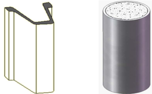
Fig. 2. Structural diagrams of a U-type steel structure and a concrete-filled steel tube.
