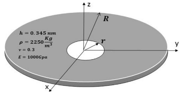
Fig. 1. Geometry of annular graphene sheet.
