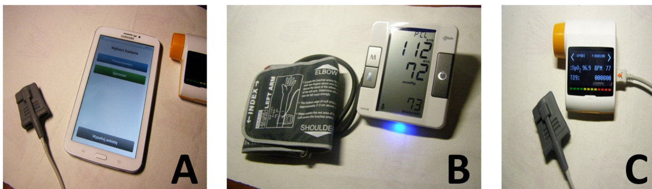
Fig. 1. Equipment used for telemonitoring: A. Mobile phone as a reporting device, B. sphygmomanometer, C. spirometer and pulse oximeter.
