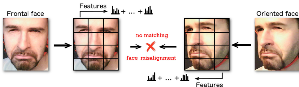
Fig. 2. Example of misalignment of the face in the presence of head pose variations.
