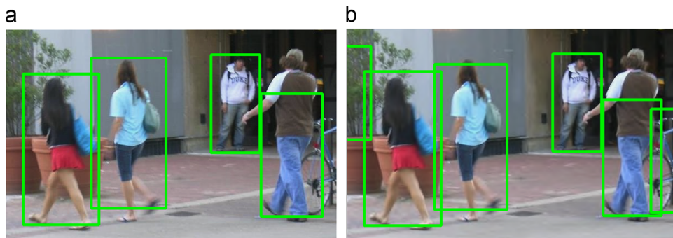
Fig. 2. “Ringing” caused by JP2 compression in (b) can occur at high spatial frequencies that are difficult for the human visual system to discern, nonetheless, the presence of this distortion is sufficient to degrade the performance of a pedestrian detection algorithm (HOG+SVM) by causing an increase in false positives.
