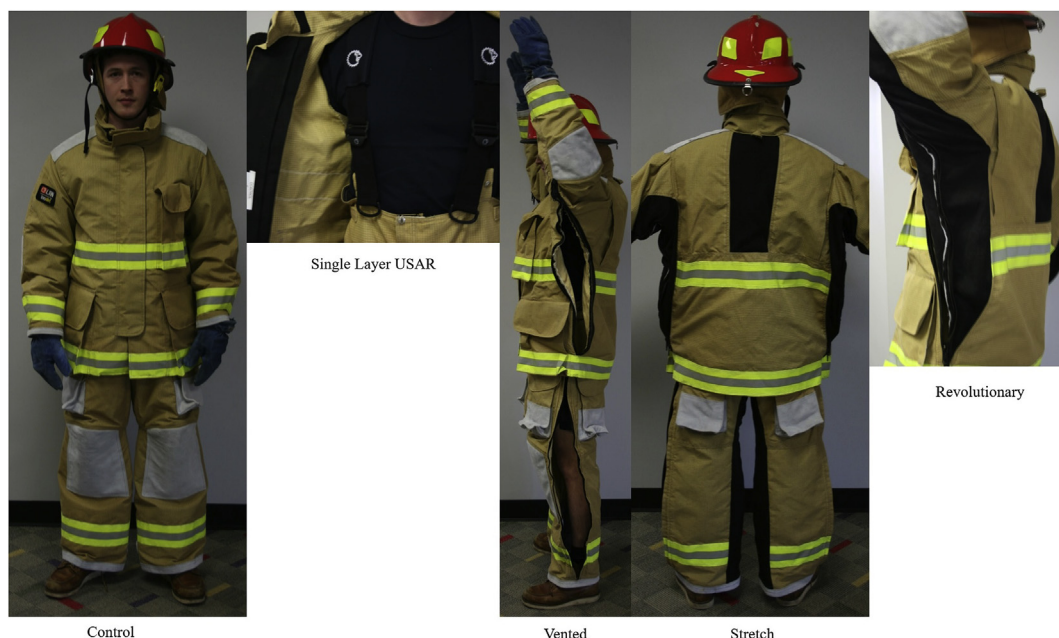
Fig. 1. Control turnout suit and developed prototype designs: single layer USAR system, Vented prototype, Stretch prototype, and Revolutionary prototype with combined designs.
