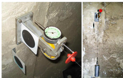
Fig. 1. The invar wire and the gauge used to remove the scale ambiguity in Scaioni et al. (2014). Reprinted by permission from: Springer Nature Earth Science Informatics (Photogrammetric techniques for monitoring tunnel deformation, M. Scaioni, L. Barazzetti, A. Giussani, M. Previtali, F. Roncoroni, M. Alba), © (2014).
