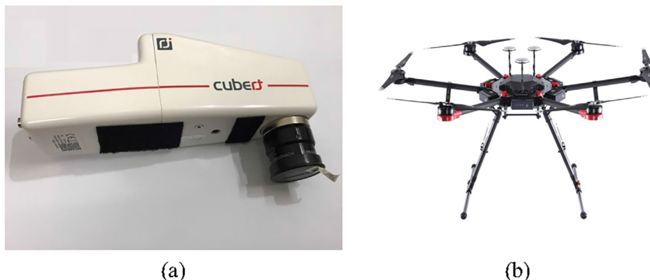
Fig. 1. Sensor system and UAV platform. (a) Cubert hyperspectral camera and (b) DJI Jingwei M600 PRO.
