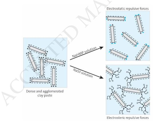
Proposed kaolinite deflocculation mechanism using NaSil and NaHMP
