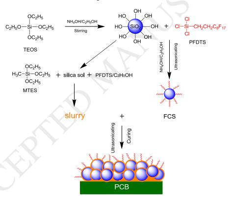
A feasible sol-gel method was developed to fabricate fluoro-functionalized colloidal silica-based superhydrophobic coating on PCB. The coating exhibits not only good waterproof, self-cleaning and anticorrosion capability, but also promising weathering resistance even in harsh environment, such as under UV irradiation or in strong acid or
