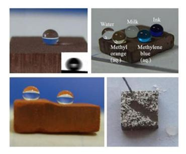
The copper-based materials have outstanding superhydrophobicity and excellent self-cleaning property. The strong repellence has universality and long-term durability/stability. Moreover, the superhydrophobicity can be regenerated once destroyed by abrasion/scratch or fouling.
