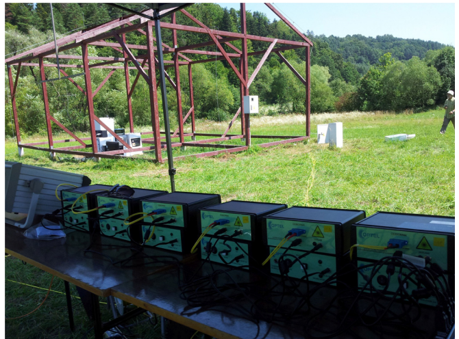
Fig. 3. Electro-optic measuring system and the test house with the LPS and typical electrical and electronic household appliances.
