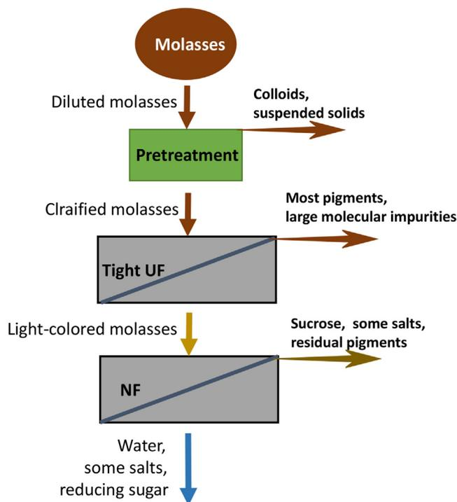
Fig. 1. Schematic diagram of molasses refining by an integrated membrane process.
