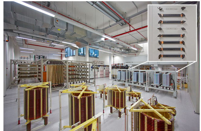
Fig. 3. Resistor and inductance setup ( R_{prim} , L_{prim} and R_{sec} , L_{sec} ) for the adjustment of the current and power factor.
