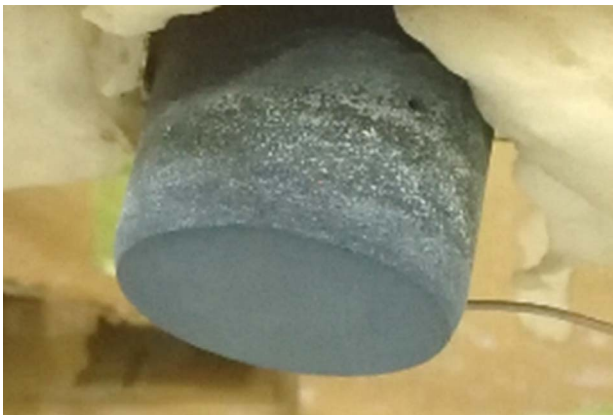
Fig. 2. Nanoparticle-deposited surface (NPDS).
