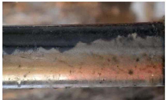
Fig. 1. Flow pattern of the liquid produced by mixing oil with water.
