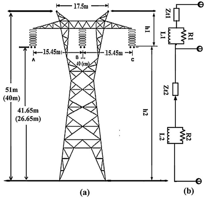
**Fig. 1.** (a) Tower configuration (values in brackets are midspan heights), and (b) multistory model of transmission tower.
