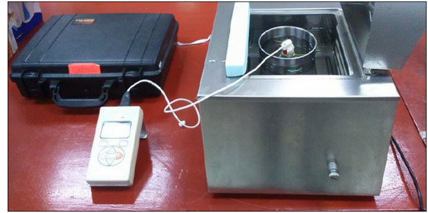
Fig. 1. KD2 Pro thermal conductivity measurement setup.
