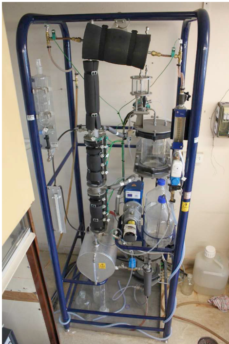
Fig. 1. The binary distillation column plant at process control laboratory.
