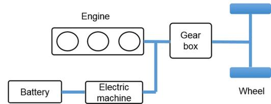
Fig. 1. Parallel mild-hybrid architecture.
