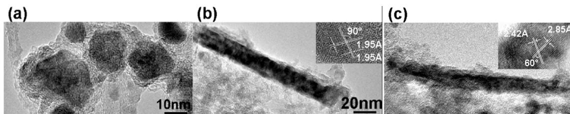
Fig. 1. HRTEM images of (a) carbon nanoparticles produced from nanosecond laser irradiation with pulse energy of 200–600 mJ, (b) carbon nanowire produced from picosecond laser irradiation with pulse energy of 65–95  $\mu$ J, (c) carbon NWs produced from femtosecond laser irradiation with pulse energy of 0.2–1.5 mJ.
