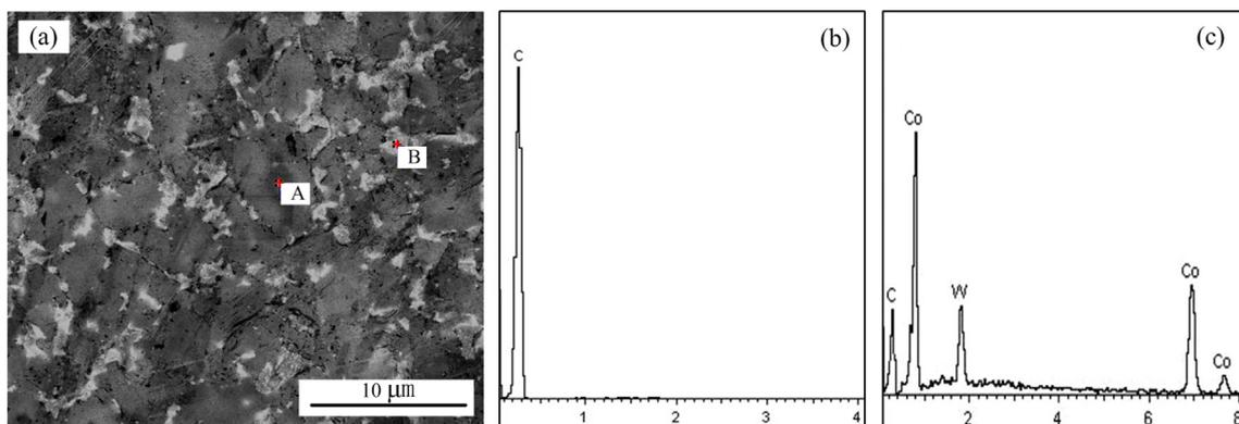
**Fig. 1.** SEM micrograph and EDX analysis of the PCD surface, (a) SEM micrograph of the polished surface, (b) and (c) EDX composition analyses marked in points A and B, respectively.
