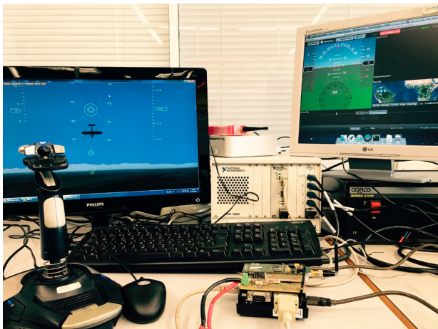
Fig. 1. Hardware in the loop simulations setup
