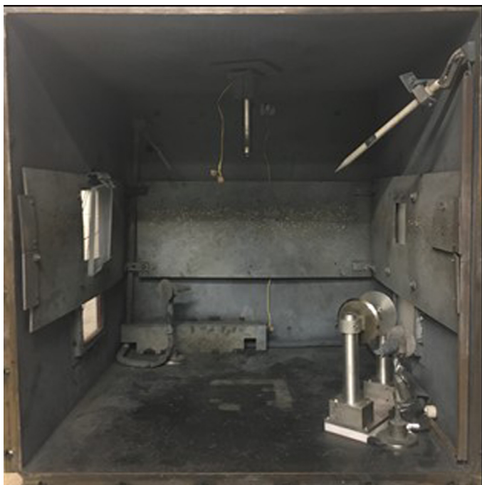
Fig. 1. The probe (bottom right corner) mounted in the 1.81 m 3 explosive blast chamber at the University of Illinois at Urbana-Champaign Explosive Diagnostics Lab.
