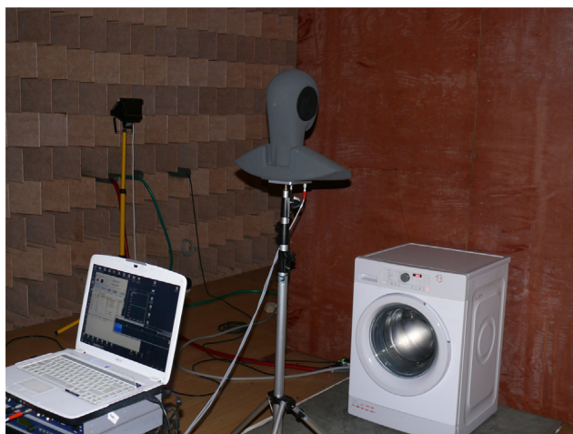
Fig. 1. Recording of washing machine sounds in semi-anechoic chamber.
