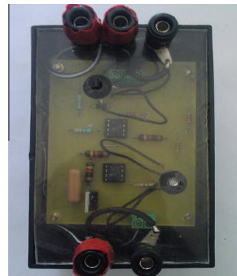
Fig. 3. Realized solar radiation and temperature sensors.
