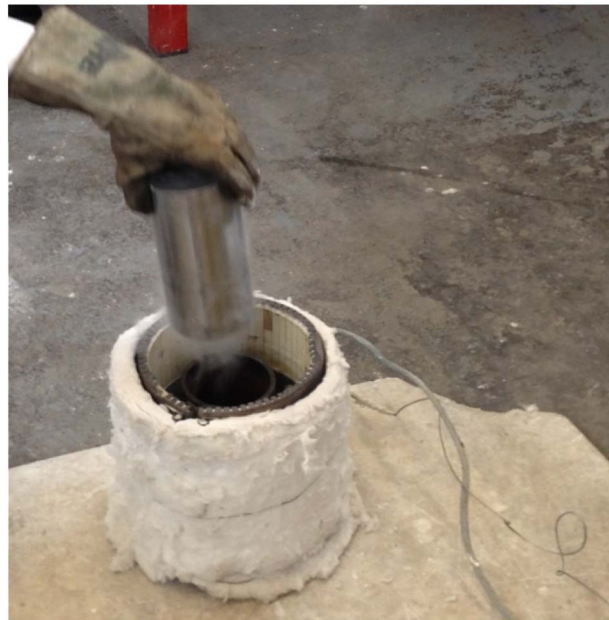
Fig. 1. Inserting the liner (AISI304) inside the heated C-Mn pipe.
