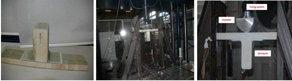
Figure: Top-hat stiffened composite panels under dynamic loading for marine structure applications.
