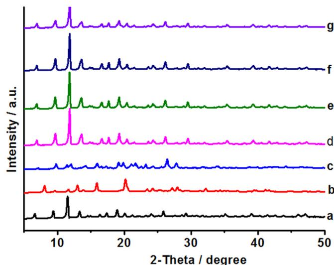
Fig. 1. The simulated XRD pattern of HKUST-1 (a). The XRD patterns of the samples synthesized in pure water at reaction time of 2 h (b) and 12 h (c). XRD patterns of  $\text{Cu}_3(\text{BTC})_2$  synthesized in water/n-hexane mixtures with oil:water volume ratio of 1:9 (d), 2:8 (e), 3:7 (f), and 5:5 (g) at reaction time of 2 h.
