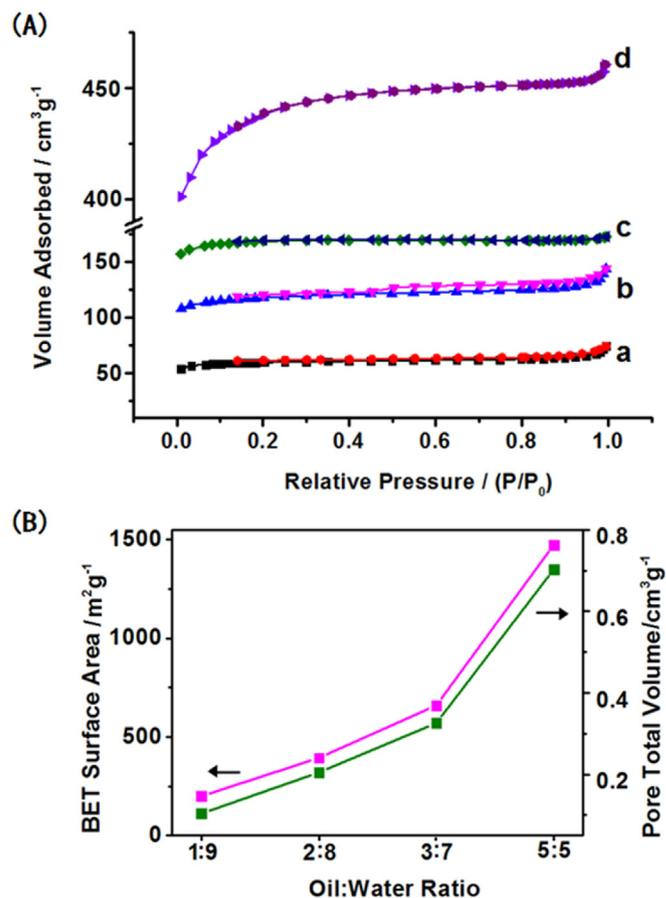
Fig. 2. A:  $\text{N}_2$  adsorption–desorption isotherms of the MOFs synthesized in water/n-hexane mixtures with oil:water volume ratio of 1:9 (a), 2:8 (b), 3:7 (c), and 5:5 (d). B: Dependence of BET surface area and total pore volume of  $\text{Cu}_3(\text{BTC})_2$  on oil:water volume ratio.
